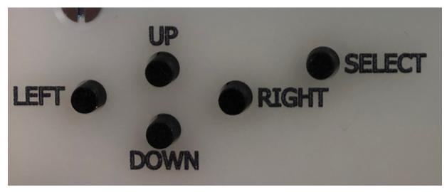
Use the **left** and **right** buttons to change the screen that is displayed. If the screen that is currently displayed includes a configuration option, its value can be changed using the **up** and **down** buttons (Note that in current versions of the Spot Demonstrator Kit firmware/sketch there are no such settings available). The new value is selected and stored to EEPROM by pressing the **select** button.
