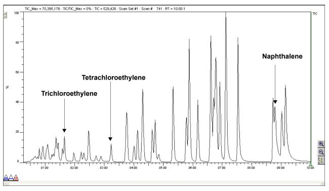
Figure 1: Example Chromatogram of the Analytes in the Restek 8260B MegaMix Standard
