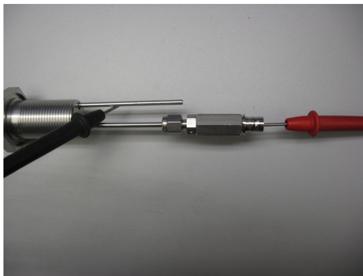
Figure 3: BNC Continuity Check
