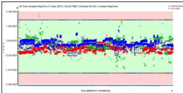
Models must be made for each implanter individually. This is due to differences in the analyzer magnet assembly and physical differences in the equipment. While this may appear like a lot of models, each tool only requires a single model and those models cover all the species processed through that analyzer magnet.
