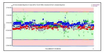
Models must be made for each implanter individually. This is due to differences in the analyzer magnet assembly and physical differences in the equipment. While this may appear like a lot of models, each tool only requires a single model and those models cover all the species processed through that analyzer magnet.
