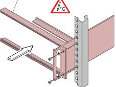
Slide the TPG500 into the rack chassis adapter ...
