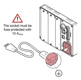
If the unit is installed in a switching cabinet, the mains voltage should be supplied and turned on via a central distributor.
