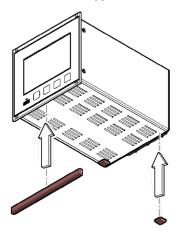
... and slip the supplied rubber bar onto the bottom edge of the front panel.
