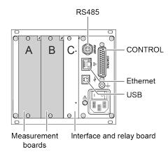
Measurement plug-in board:
