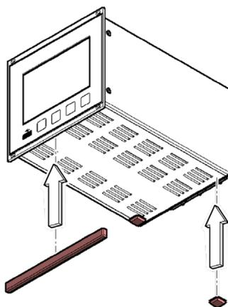
... and slip the supplied rubber bar onto the bottom edge of the front panel.
