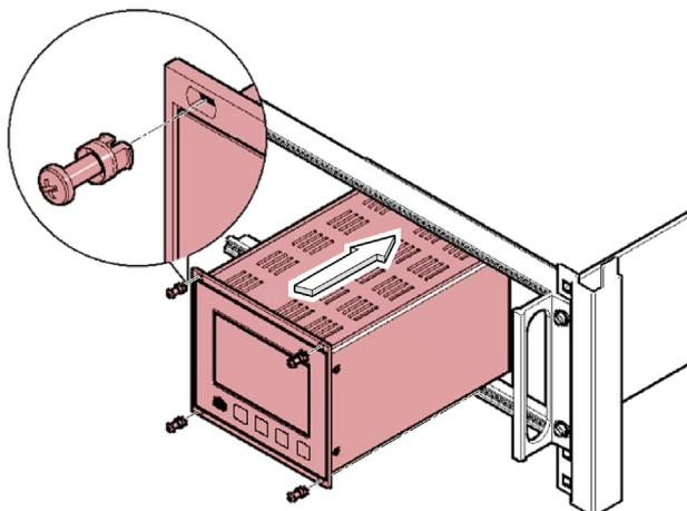
... and fasten the adapter panel to the rack chassis adapter using the screws supplied with the TPG500.
