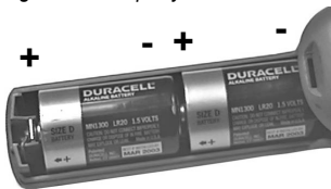
Figure 1. Properly Installed Alkaline Batteries
