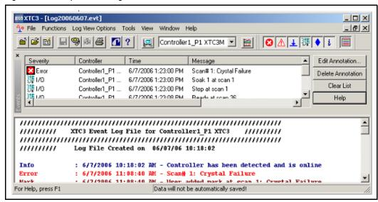
Log files contain Errors, Warnings, Events, I/O Events, Marks, and Informational messages. It is possible to selectively display or hide these classes of events or to color code them to facilitate locating errors, etc. **The Log View Options** menu and **Log View Toolbar**, shown in Figure 4-21, controls these options.
