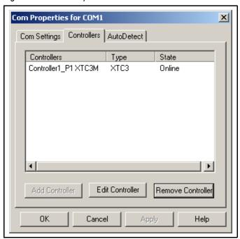
The **Controllers** tab (refer to Figure 2-11) allows for a Controller to be removed (using the **Remove Controller** button) or edited (using the **Edit Controller** button). When editing the Controller, changes can be made to the **Controller Name**, which is used to identify the Controller in the software. The **AutoDetect** tab (see Figure 2-12) allows XTC/3 Editor communications to streamline the detection of a controller at a serial port.
