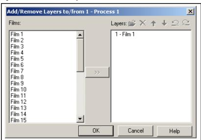
To add a layer(s), select the film(s) in the **Films** side and press the >> button. The corresponding layer(s) will then appear in the **Layers** side. (See Figure 3-19.)
