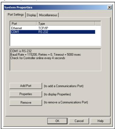
For Serial Communications (RS-232), the port properties can be changed by selecting the serial port item (e.g. COM1), then clicking the **Properties** button on the **Port Settings** page (See Figure 2-9). Clicking the **Properties** button will display the **Com Properties** page with three tabs shown in Figure 2-10 and described in section 2.2.2.
