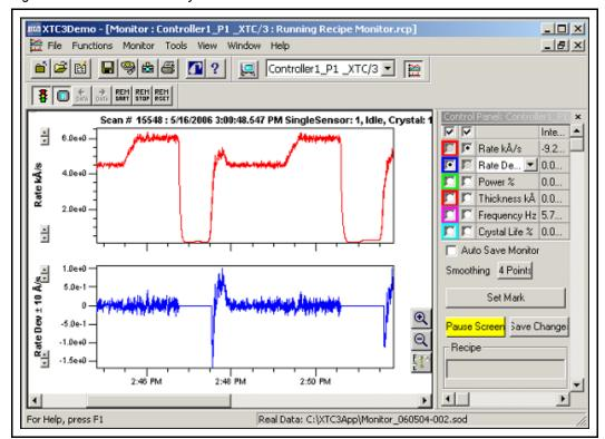
Data collection from the XTC/3 is done for six data parameters. Only two data parameters can be displayed on the **Trend Graph**. The display parameter choice is made from radio buttons on the grid of the Control Panel as shown in Figure 4-3.
