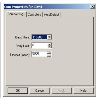
The **Baud Rate** is set by default to 115200 for RS-232 communications. This is the fastest rate possible (at this time) in the XTC/3 Controller.
