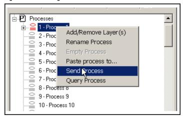
A process can be filled or replaced with the content of a process from the controller via Query Process. Select a process, right click to bring up the context menu, select **Query Process**. See Figure 3-30.
