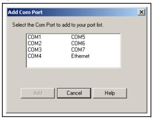
If communicating to the XTC/3 Controller via **RS-232**, select the port to which the **serial cable** is connected. After selecting the correct port, click the **Add** button. If communicating to the XTC/3 Controller via **Ethernet**, select the Ethernet port and press **Add**. The **System Properties** dialog and will now display the added ports as shown in Figure 2-5.
