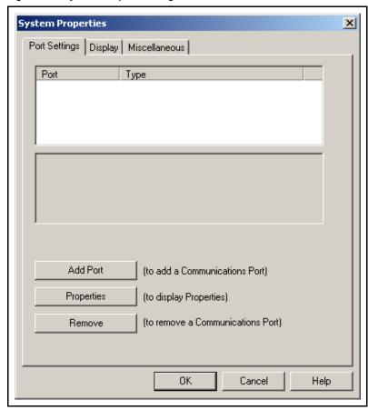
Three buttons are provided on the Port Settings tab which affect the port highlighted in the list: **Add Port**, which is described in section 2.2.1 on page 2-4, **Properties** for Serial communications and **XTC3 Controller List** for Ethernet communications, which is described in section 2.2.1 on page 2-4, and **Remove**, which deletes the port and any associated parameters from the System Properties.
