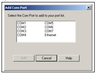
**NOTE:** Communication problems often occur when other programs (for example, PDA link programs) that either actively use the communications port, or wait for activity on the communications port, are running in the background. These types of programs should be disabled or removed from the computer used for XTC/3 Editor communications.
