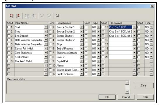
I/O functions can be assigned to their respective input (1 to 9) or output (1 to 20) using a drop-down list, see Figure 3-15. These I/O functions are described under the **Input Names**, **Relay Names**, and **TTL Names** columns. If **Sel Process** input or a **Cruc Src** output is chosen, a varying number of inputs/ouputs is reserved. The reserved slots will be grayed out and cannot be sent or queried (see input 7 or 14/15 TTL Send above or Relay 4-9 in Figure 3-13).
