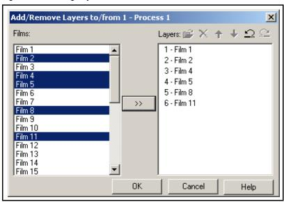
If there are already layers, add new layers at a certain position by selecting the position and clicking the >> button. For example, as shown in Figure 3-20 and Figure 3-21, Films 12 and 15 are inserted above Film 5, position 4.
