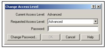
When changing from **Normal** level to **Advanced** level, enter the correct password in the **Password**: field and click **OK**. To change a Password, click the **Change Password...** button, enter the old Password and the new Password in the appropriate boxes, and click **OK**. As with any password, it should be remembered and protected.
