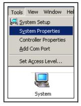
The first time the XTC/3 Editor is run it starts on the **System Setup Screen** and prompts for a communications port (Com Port) to be configured. See Figure 2-2. From this dialog, select and add the Com Port to be used for communications with the XTC/3 Thin Film Controllers.
