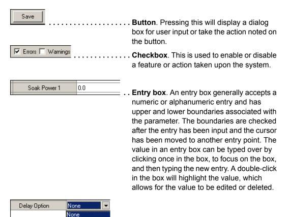
**Pulldown**. A pulldown, indicated with a downward triangle, provides a list of acceptable inputs for the parameter. A highlight is used to select the parameter. Some entry boxes that use pulldowns can also be directly edited.
