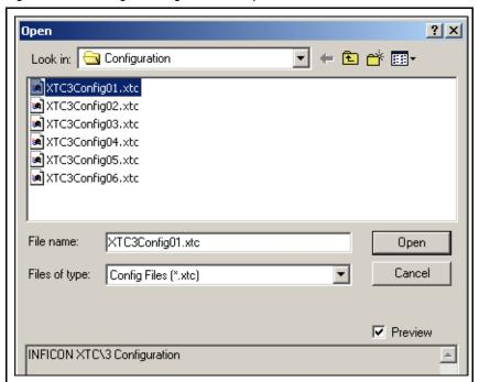
If the **Files of type** box does not show a XTC/3 Configuration (\*.xtc) or All Files (\*.\*), then click on the pulldown and select one of these types from the list. Clicking on a filename will display a few lines of text in the preview box which describe the Configuration. Once a file is selected and opened, the main window of the **Configuration Editor** will be displayed (see Figure 3-8).
