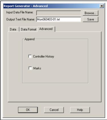
When the desired options are selected, click **Save** to write the data to the output file. The files generated are plain text files and can be viewed with any text editor, such as Notepad, and imported into other programs such as Excel.
