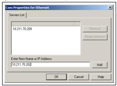
After typing the IP address of the XTC/3 instrument, click on **Add**. The Controller's IP Address is then added to the list.
