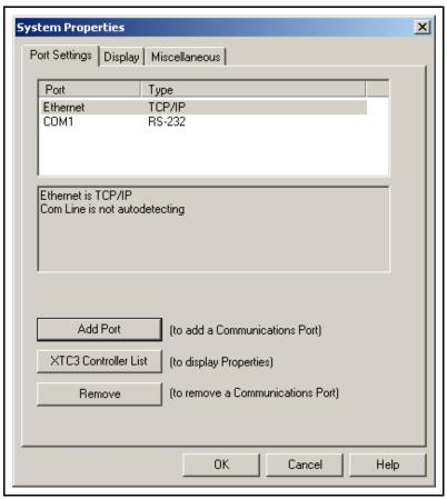
The IP address of each XTC/3 instrument connected to the Ethernet network (in the form xxx.xxx.xxx.xxx) can be added by first selecting the Ethernet item on the ports list of the Port Settings page and then pressing the **XTC3 Controller List** button. A **Com Properties for Ethernet** box will open (see Figure 2-6).
