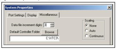
Data file increment digits . . . . . . This entry configures the number of numerical places used in the file name index for SOD (data) files. For example, selecting 3
