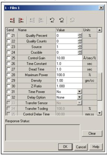
To edit any parameter, enter the desired value in the **Value** column or use the corresponding pulldown or spinner. Any parameter can be sent to the XTC/3 Controller by selecting the parameter in the **Send** column and pressing the **Send Selection** button. The entire set of parameters can be sent by pressing the **Send All** button (regardless of the **Send** column selections). The **OK** button will save all changes to the Editor memory; the **Cancel** button will discard all changes.
