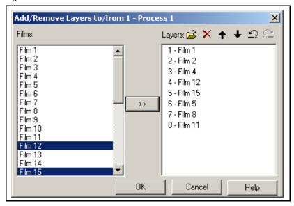
A layer (on the right side) can be moved up or down by first selecting it and either dragging it up or down with the mouse or by clicking the up or down arrow in the toolbar located above the Layers side. In the example shown in Figure 3-22, Film 11 is moved up to the positon above Film 4. The result is shown in Figure 3-23.
