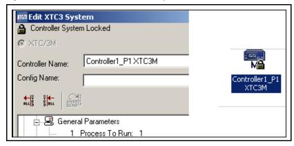
If either File >> Edit Configuration or the Configuration Editor icon is selected to start the Editor, then the dialog shown in Figure 3-6 will be displayed. This allows for a Controller to be specified as the target for a new or existing Configuration. To
