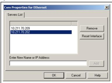
Clicking on the **Reset Interface** button resets the Controller's Ethernet parameters to their default values.
