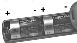
Figure 1. Properly Installed Alkaline Batteries
