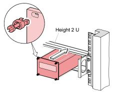
$\dots$  and fasten the PGD500 to the rack chassis adapter using collar screws and plastic sleeves.
