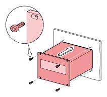
... and secure it with four M3 or equivalent screws.
