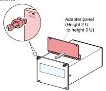
Slide the PGD500 into the rack chassis adapter ...
