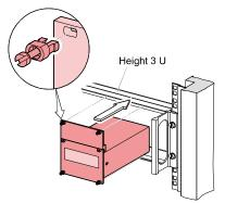
...and fasten the adapter panel to the rack chassis adapter using collar screws and plastic sleeves.
