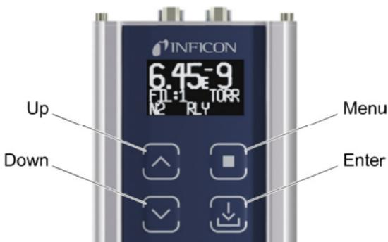
There are four soft-keys located on the front panel, below the display. These keys are used to select and program the various functions available. During programming of the BAG302, the display will identify what each function key represents.
