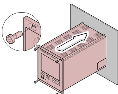
... and secure it with four M3 or equivalent screws.
