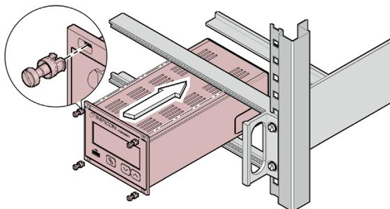
... and fasten the VGC501 to the rack chassis adapter using the screws supplied with it.
