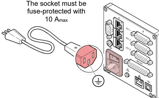
If the unit is installed in a switching cabinet, the mains voltage should be supplied and turned on via a central distributor.
