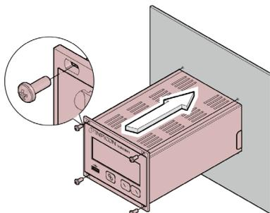
... and secure it with four M3 or equivalent screws.
