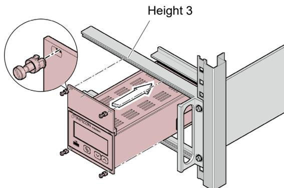
... and fasten the adapter panel to the rack chassis adapter using the screws supplied with the VGC501.
