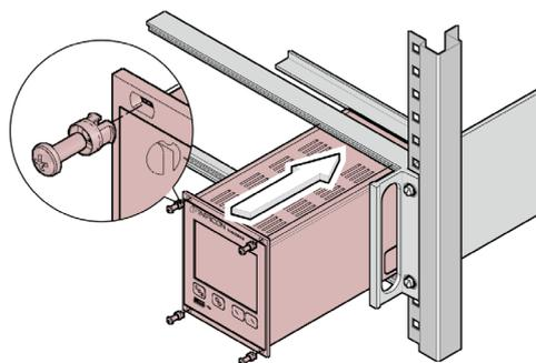
... and fasten the adapter panel to the rack chassis adapter using the screws supplied with the VGC502/503.
