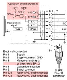
2 Connect the sensor cable to the gauge and the control-
