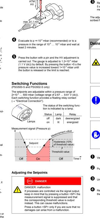
R The status of the relay and lamp is not affected by pressing the button
