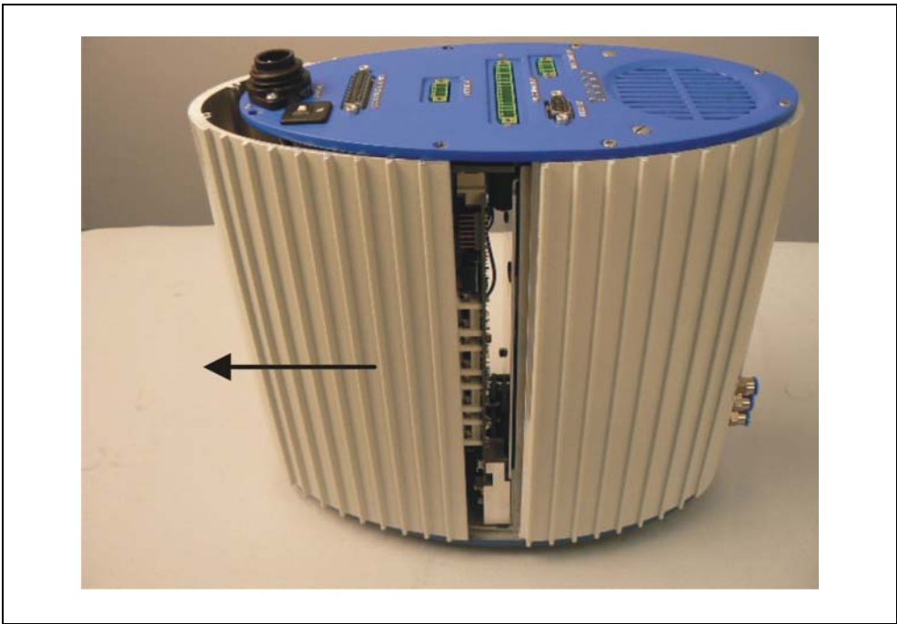
Fig. 7-6 Open the front part of the housing like the arrow indicates
