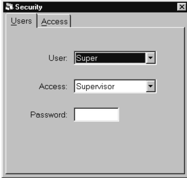
**User:** Drop down used to select an existing user, to edit their Access or Password. It is not possible to edit or add a user name in the User drop down. Use the New SoftKey to create a new User. Use the Delete SoftKey to delete the selected user.
