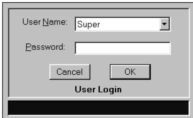
**Note:** The SQS-242 software ships with one pre-assigned user. The user name is Super, with no Password. Do not confuse this with the registration Name and Unlock Code discussed in the previous section.
