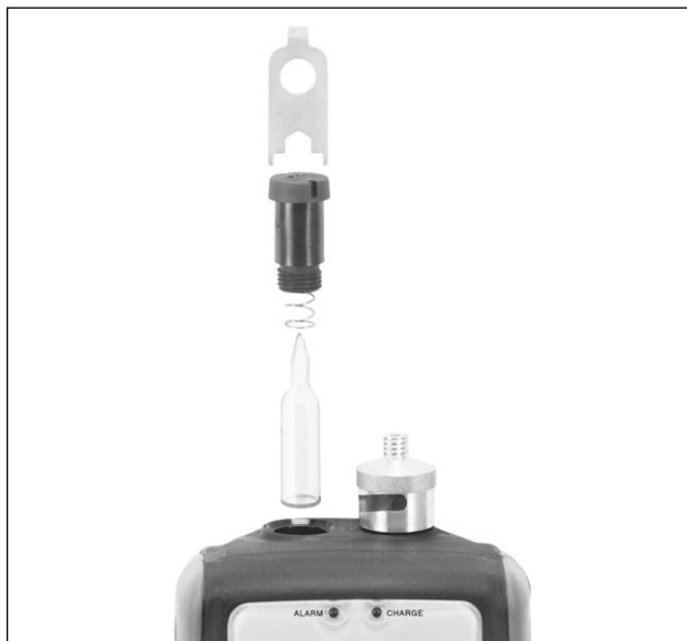
Figure 21. Removing the UV Lamp
