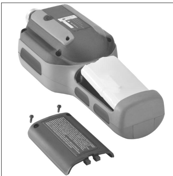
Figure 4. Battery Pack Removal and Replacement
