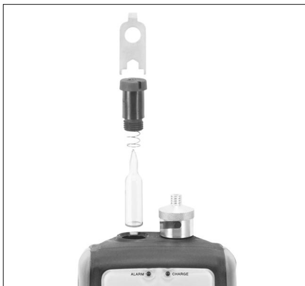
Figure 27. Removing the UV Lamp
