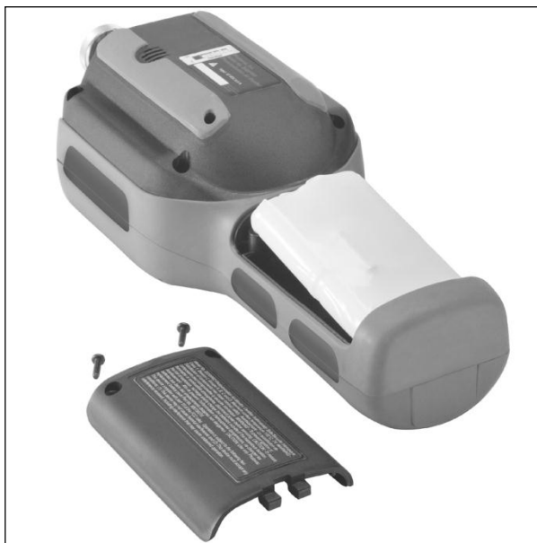
Figure 4. Battery Pack Removal and Replacement
