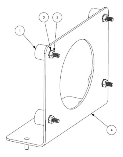
The mounting bracket may be positioned in any orientation and mounted to any surface, other than a wall or ceiling, able to withstand the combined weight of IMM-100 and the mounting bracket (approximately 0.68 kg (1.5 lbs.)).
