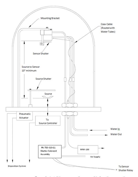
Generally, install the sensor as far as possible from the evaporation source (a minimum of 25.4 cm (10 in.) is recommended) while still being in a position to accumulate thickness at a rate proportional to accumulation on the substrate. Proper sensor placement positions the face of the crystal normal to the evaporation source, is within the material flux plume, and is not obstructed from a line of sight to the source.
