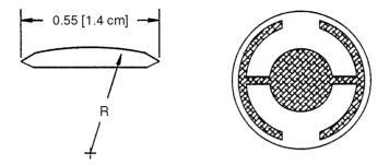
The lowest frequency response is primarily a "thickness shear" mode that is called the fundamental. The characteristic movement of the thickness shear mode is for displacement to take place parallel to the major monitor crystal faces. In other words, the faces are displacement antinodes.
