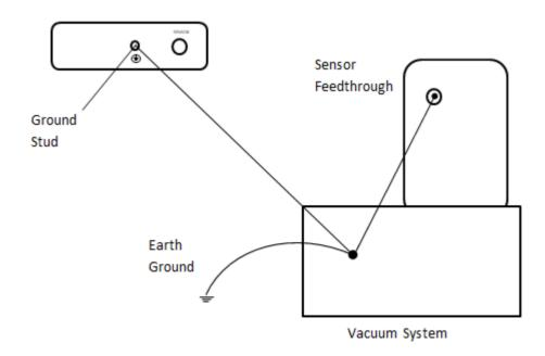
2. The instrument is also connected to earth ground through the 24 V power cable. The power supply is in turn connected to earth ground by the sealed three conductor power cable, which must be plugged into a socket outlet with a protective earth ground terminal. Extension cables must always have three conductors including a protective earth terminal.
