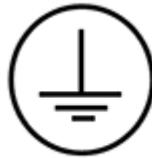
This symbol indicates where the protective earth ground is connected inside IMM-100. Never unscrew or loosen this connection.
