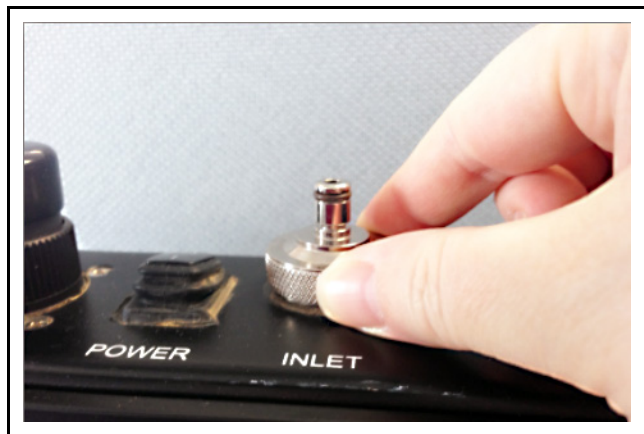
Figure 5-1 Unscrew the inlet filter housing
