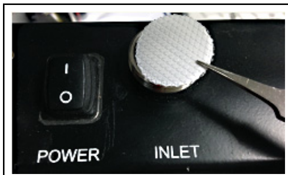
Figure 5-2 Replacing the inlet filter
