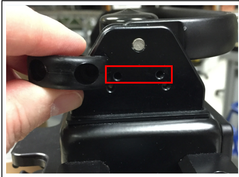
Figure 2-18 Shoulder strap adapter shown next to holes in the handle
