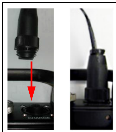
Figure 2-24 Connecting the charger adapter
