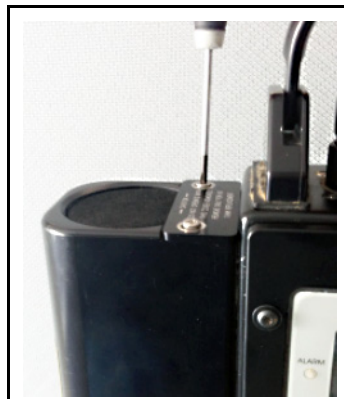
Figure 2-44 Replace the hydrogen fuel cylinder retention plate
