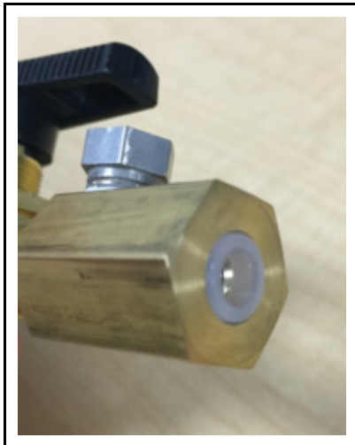
Figure 5-13 Fully inserted Hydrostik adapter seal
