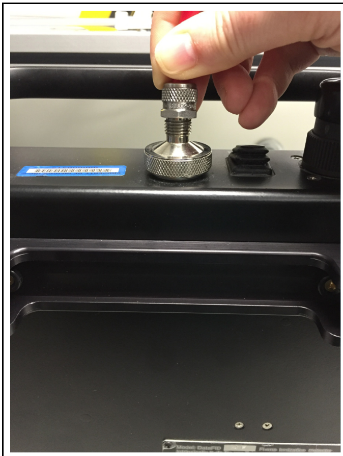
Figure 2-12 Attach telescoping probe
