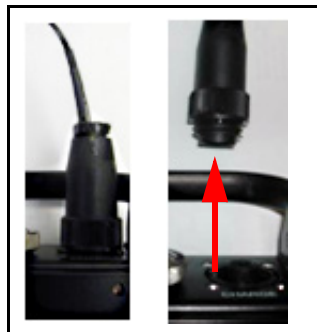
Figure 2-25 Disconnect the charger adapter
