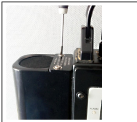
Figure 2-40 Remove hydrogen fuel cylinder retention plate
