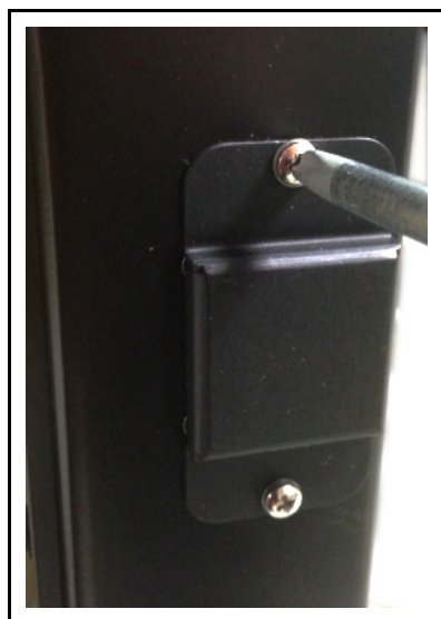
Figure 5-4 Remove exhaust cover
