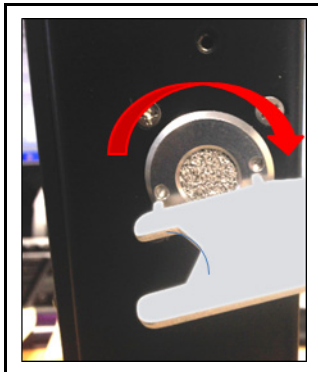
Figure 5-7 Replace exhaust frit filter and housing
