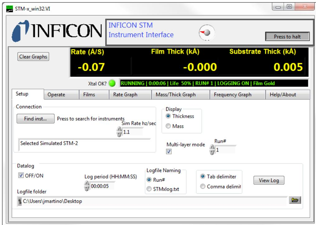
**Change Film** This option changes the active film. Clicking this opens the **FilmPicker.vi** window that displays the films to run. The existing thickness is not zeroed and the thickness is recalculated with the new Z-ratio and tooling.
