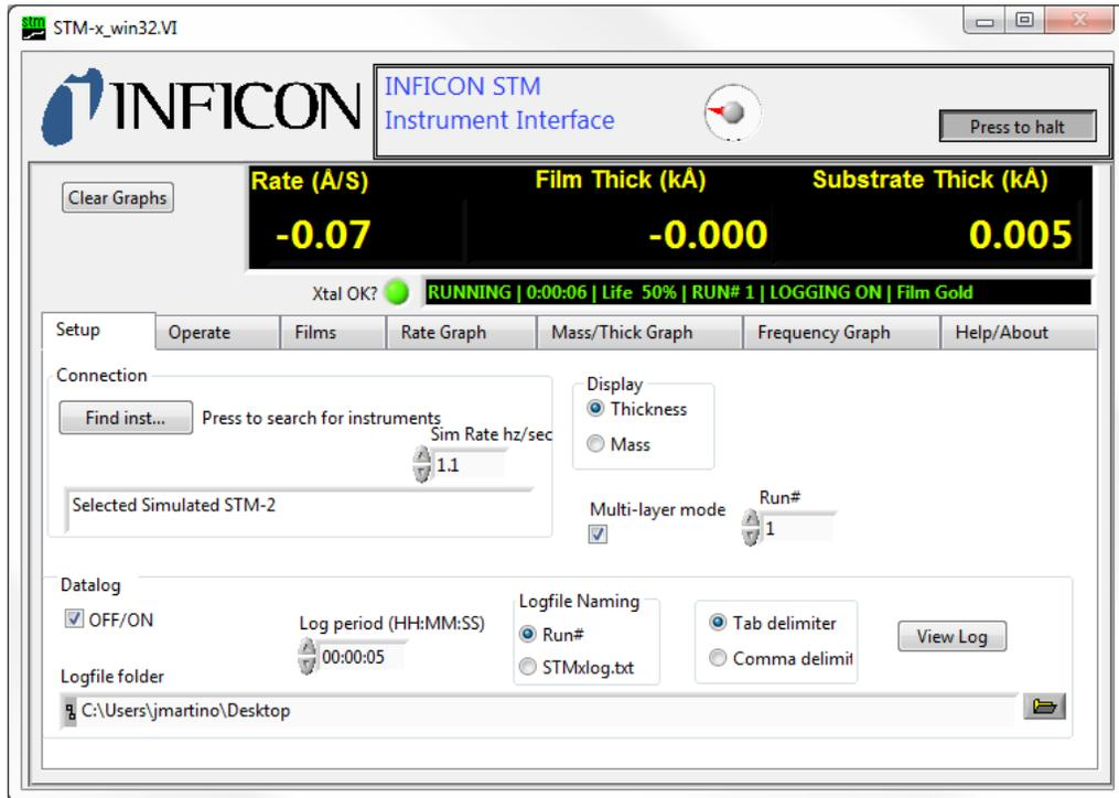
With a rate of hertz per second defined, the software converts the change in frequency to a rate in angstroms per second or microgram second per centimeter squared based on the selection of **Thickness** or **Mass** on the **Display** pane.
