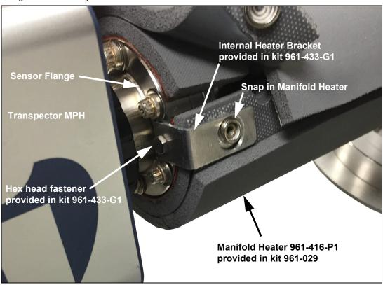
Figure 1-17 Heater jacket mount kit installation
