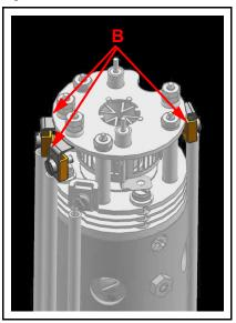
**3** Carefully pull the filament assembly from the ion source.
