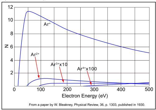
The appearance potential (i.e., the minimum electron energy required to produce a specific ion) for Ar<sup>+</sup> is 15.7 eV. The number of argon ions produced rises steeply with energy until a maximum is reached at about 55 eV. As the electron energy rises above this level, the rate of Ar<sup>+</sup> production slowly decreases.
