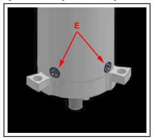
**5** Gripping the bottom of the EM assembly, gently remove the EM from the sensor assembly.
