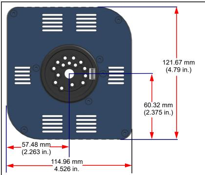
Figure 1-5 Electronics module dimensions
