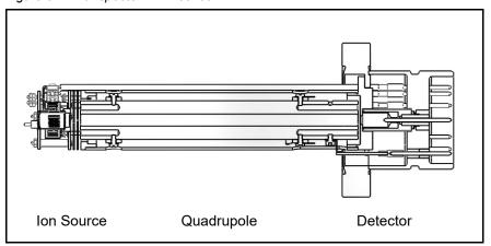
The sensor works only in a high-vacuum environment because the ions, once created, must not collide with neutral gas species or the walls of the ion source. Otherwise, they cannot be detected. At low pressure, the total flight path of the ions is long enough to pass through the quadrupole without collisions.
