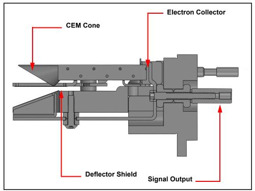
In CDEM/FC detectors, the EM cone amplifies the electron pulse, significantly increasing the analyzer's sensitivity.
