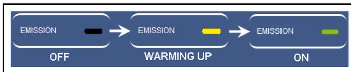
The Electron Multiplier is controlled the same way as the emission. To turn the Electron Multiplier on or off, click **EM**. There are only two different EM states: **OFF (Black)** and **ON (Green)**. See [Figure 5-11](#).
