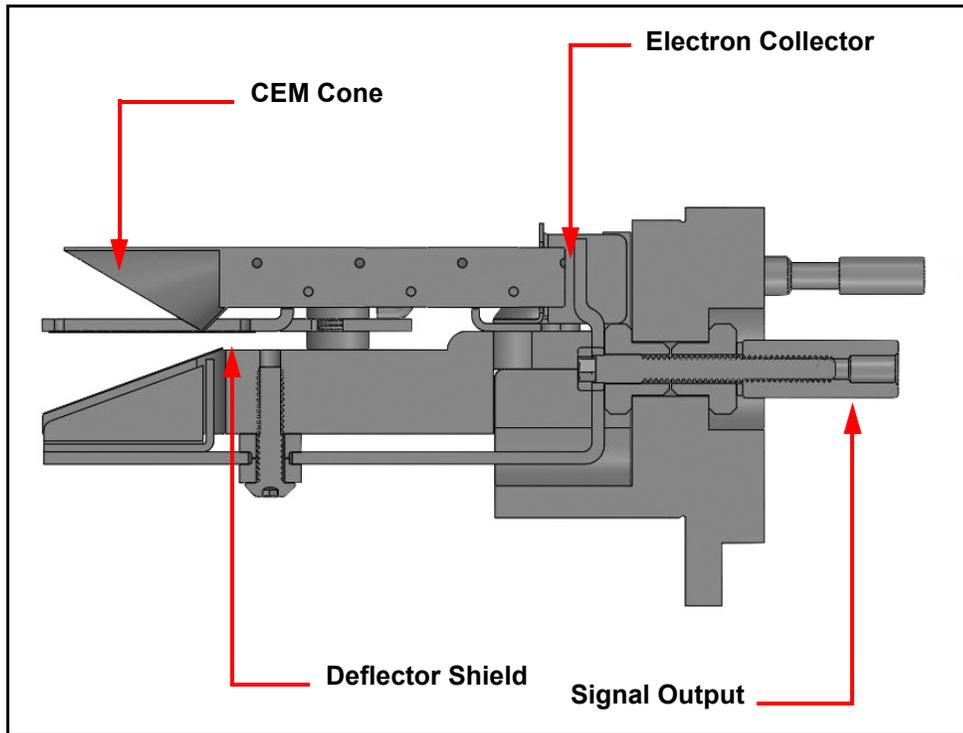
In CDEM/FC detectors, the EM cone amplifies the electron pulse, significantly increasing the analyzer's sensitivity.
