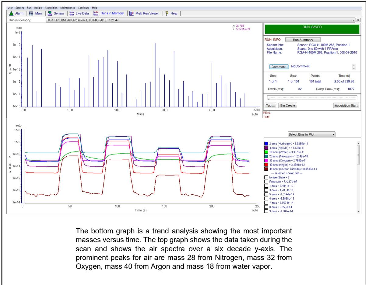
The bottom graph is a trend analysis showing the most important masses versus time. The top graph shows the data taken during the scan and shows the air spectra over a six decade y-axis. The prominent peaks for air are mass 28 from Nitrogen, mass 32 from Oxygen, mass 40 from Argon and mass 18 from water vapor.
