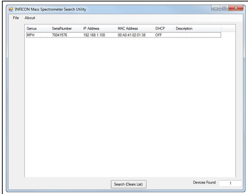
When the IMSSU first opens, nothing will be displayed. The IMSSU detects all Transpector MPH installed on the network regardless of IP address. The IMSSU will start automatically, or it can be manually started by clicking **Search (Clears List)**. The IMSSU will then display the:
