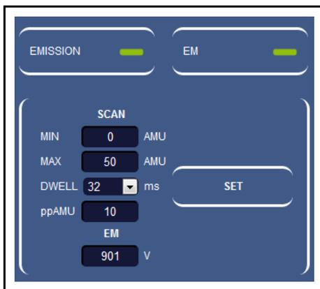
To turn On/Off Emission, click **EMISSION**. There is an indicator on the right side of the **EMISSION** button. This indicator changes color based on emission state. There are three colors, as shown in [Figure 5-10](#).
