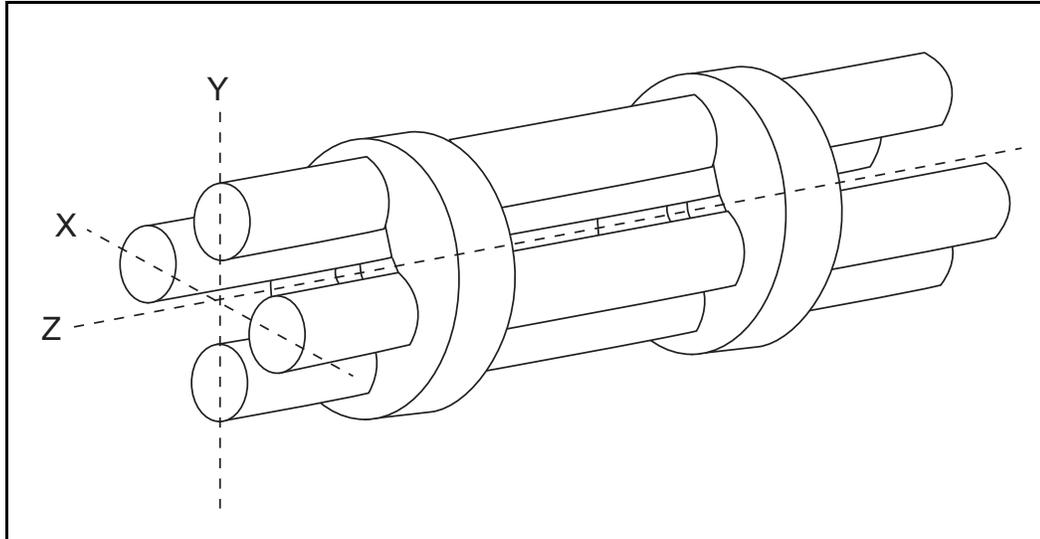
The mass filter's four rods are alternately charged to direct ions of specific masses down through the center, deflecting all larger and smaller masses (hence the term mass filter).
