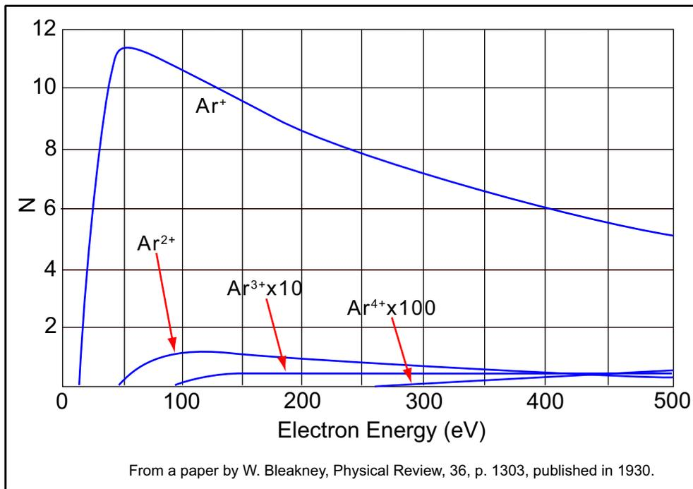
The appearance potential (i.e., the minimum electron energy required to produce a specific ion) for  $\text{Ar}^+$  is 15.7 eV. The number of argon ions produced rises steeply with energy until a maximum is reached at about 55 eV. As the electron energy rises above this level, the rate of  $\text{Ar}^+$  production slowly decreases.
