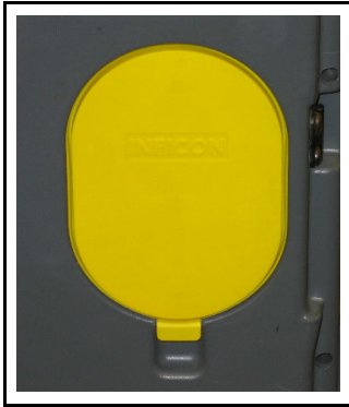
Figure 2-38 Remove the Yellow Plastic Protective Cover on the Bottom of the HAPSITE
