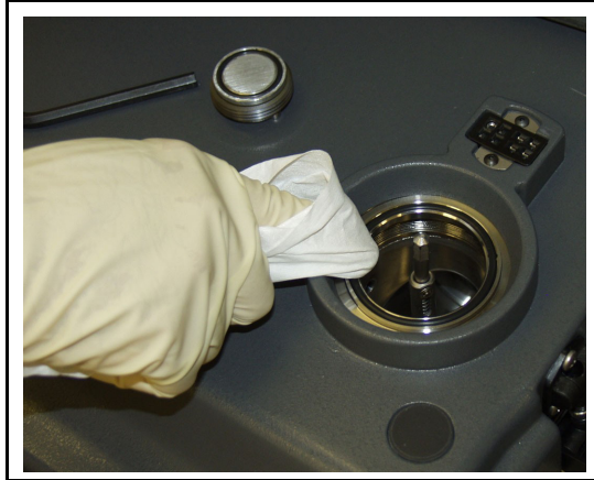
Figure 15-29 Cleaning the Service Module Rubber O-ring using a Lint-free Wipe
