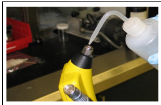
Figure 16-1 Pouring Methanol into Probe and Probe Line
