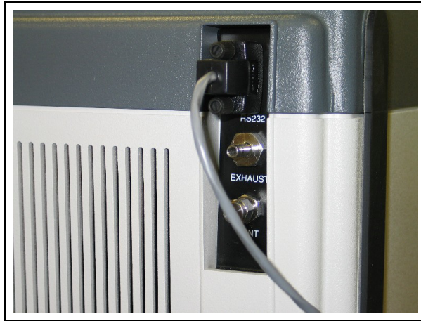
Figure 2-33 RS-232 Communication Cable Attached to Back Right Side of Service Module
