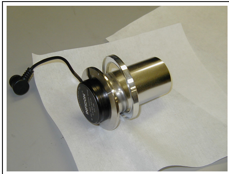
Figure 16-31 Aluminum Gasket on NEG Pump
