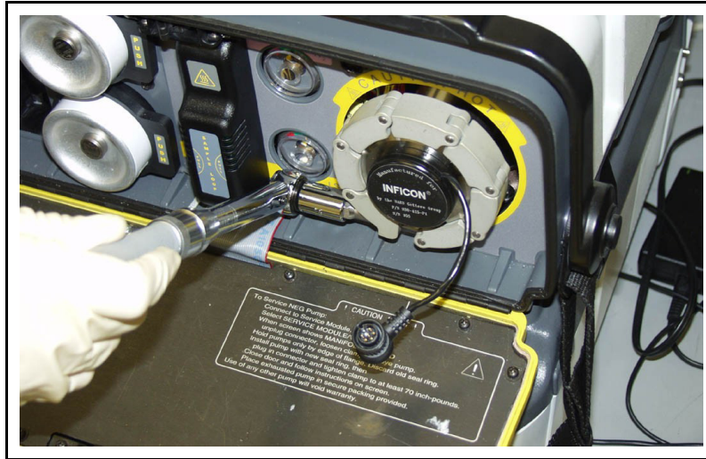
Figure 16-33 Torquing Chain Clamp
