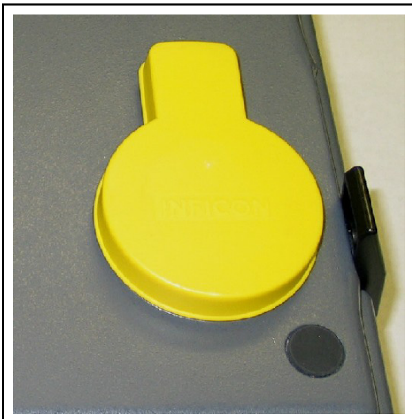
Figure 15-34 Yellow Protective Cover Placed Over Aluminum Storage Plug on Service Module
