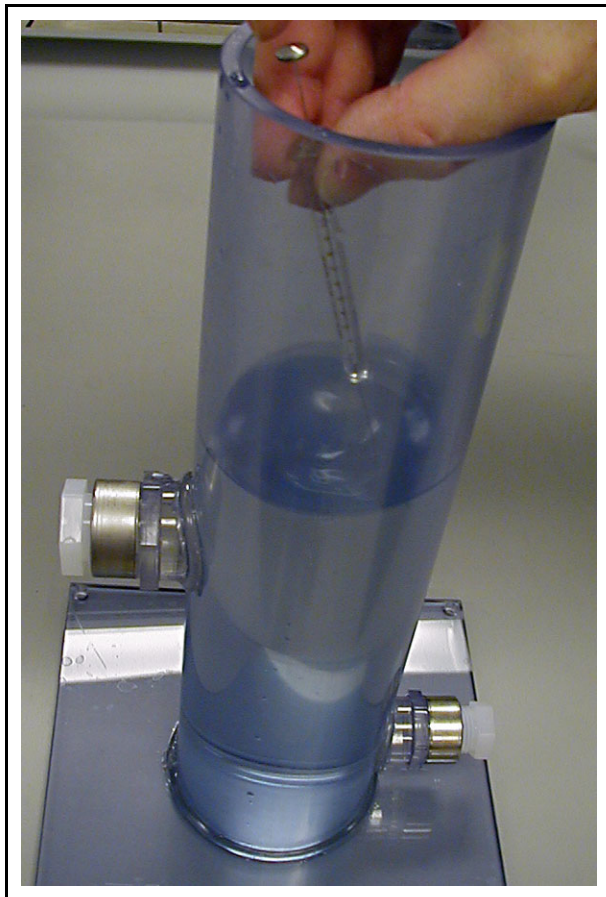
Figure 14-5 Standard spiking into a purge vessel.
