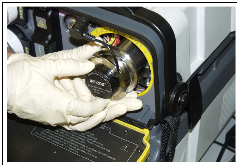
Figure 16-32 Installing New NEG Pump
