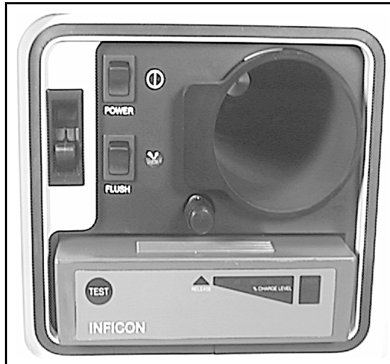
Figure 13-9 Flush Switch Inside The Headspace Instrument
