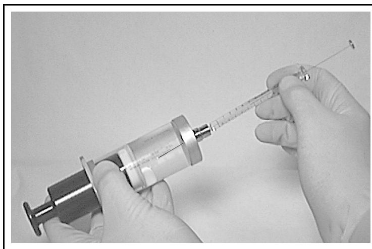
Figure 13-6 Injecting the Mix into the Sample Syringe
