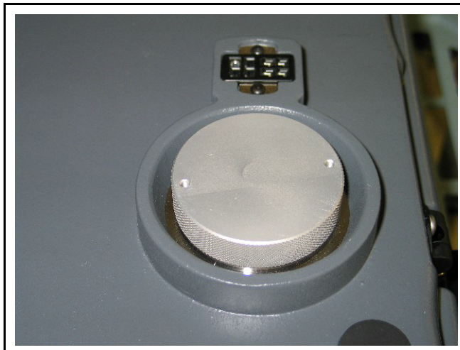
Figure 15-30 Service Module Aluminum Storage Plug in Place
