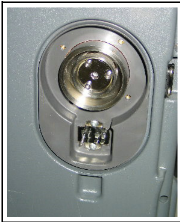
Figure 2-39 Yellow Plastic Protective Cover Removed from the Bottom of the HAPSITE
