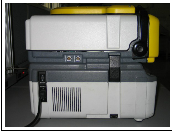
Figure 2-41 HAPSITE Attached to Service Module using Service Module Latches - Left Side View
