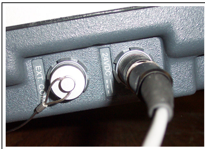
Figure 2-21 Power Supply to HAPSITE from AC To DC Power Converter
