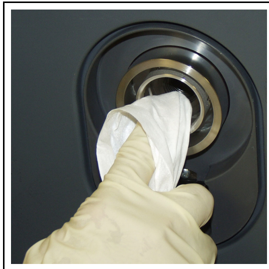
Figure 16-23 Cleaning Bottom of Manifold
