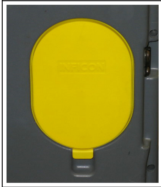
Figure 15-28 Placing Yellow Protective Cover on Bottom of HAPSITE
