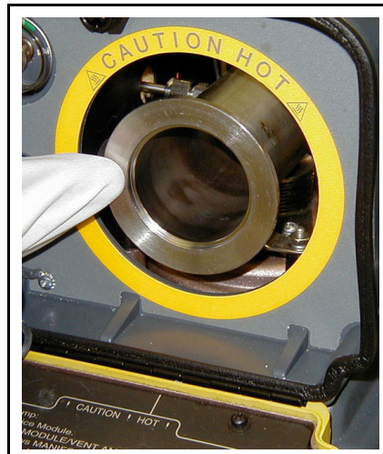
Figure 16-26 Cleaning Manifold Flange
