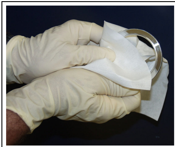
Figure 16-28 Cleaning Aluminum Gasket
