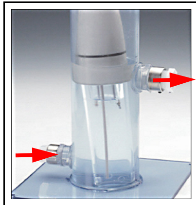
Figure 2-49 Purge Vessel Water Flow Direction Shown
