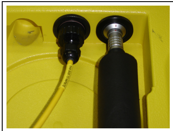
Figure 2-11 Attaching the LEMO Connector on the Probe Line to the HAPSITE
