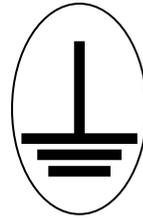
**This symbol indicates where the protective earth ground is connected inside XTC/3. Never unscrew or loosen this connection.**
