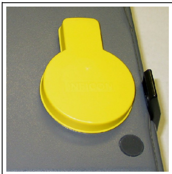
Figure 14-40 Yellow Protective Cover Placed Over Aluminum Storage Plug on Service Module
