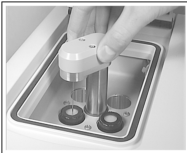
Figure 3-59 Loading the Wells
