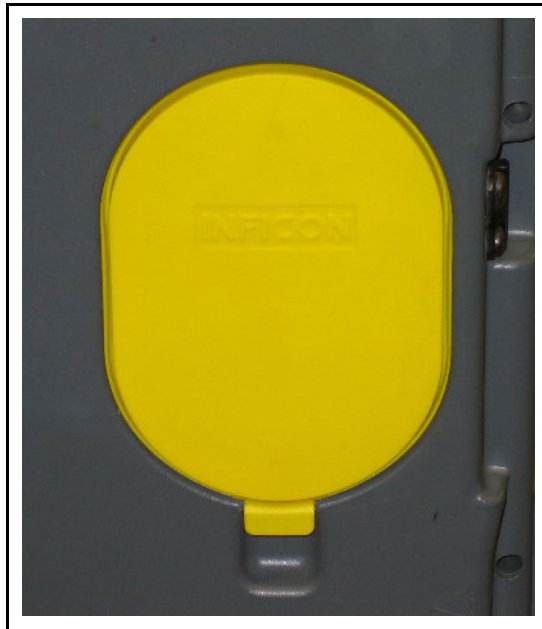
Figure 14-34 Placing Yellow Protective Cover on Bottom of HAPSITE
