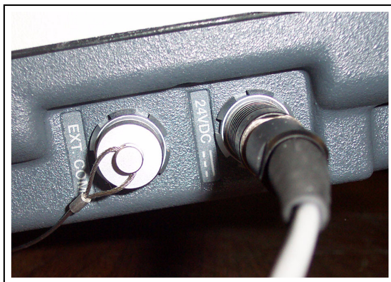
Figure 2-17 Power Supply to HAPSITE from AC To DC Power Converter
