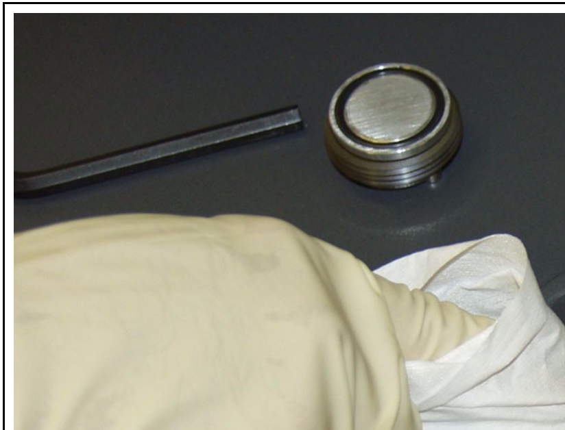
Figure 14-35 Cleaning the Service Module Rubber O-ring using a Lint-free Wipe
