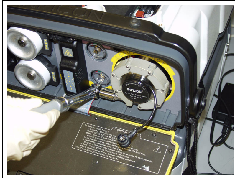
Figure 15-29 Torquing Chain Clamp
