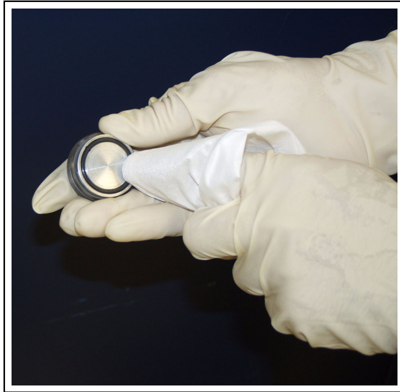
Figure 15-18 Cleaning VI Valve O-ring
