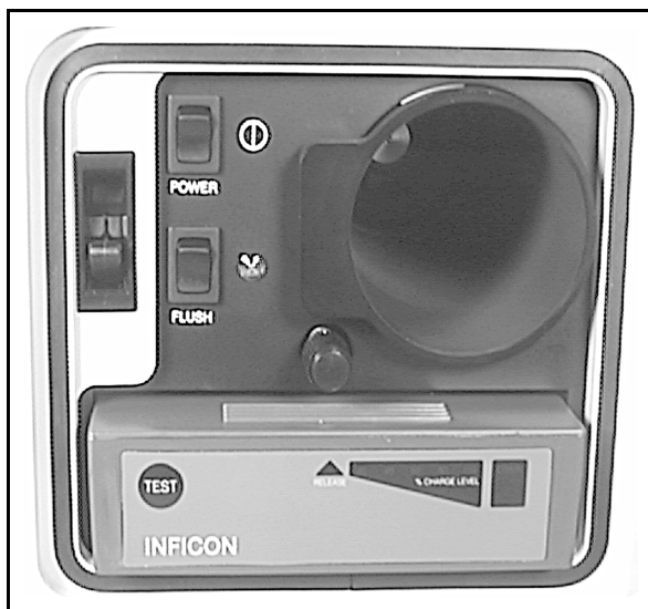
Figure 13-9 Flush Switch Inside The Headspace Instrument
