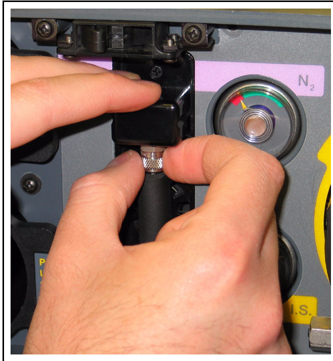
Figure 2-39 Tightening the Top Nut
