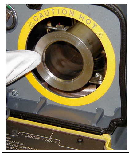
Figure 15-22 Cleaning Manifold Flange
