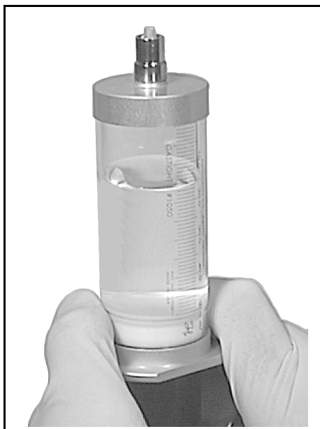
Figure 13-5 Clearing the Air Bubble from the Sample Syringe
