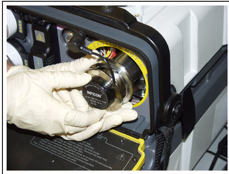
Figure 15-28 Installing New NEG Pump
