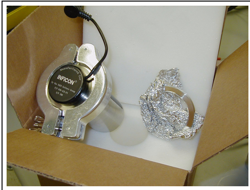
Figure 15-23 New NEG Pump and Aluminum Gasket
