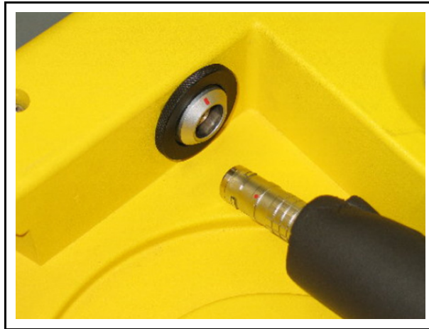
Figure 2-7 Attaching the LEMO Connector on the Probe Line to the HAPSITE
