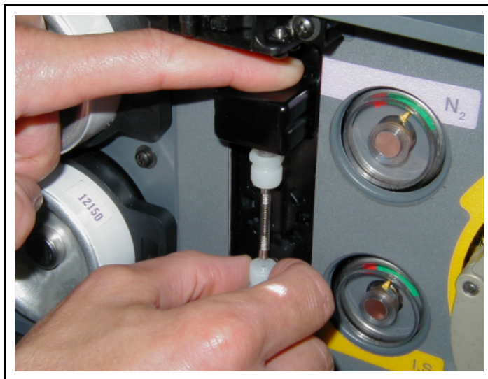
Figure 2-47 Tighten Bottom Nut
