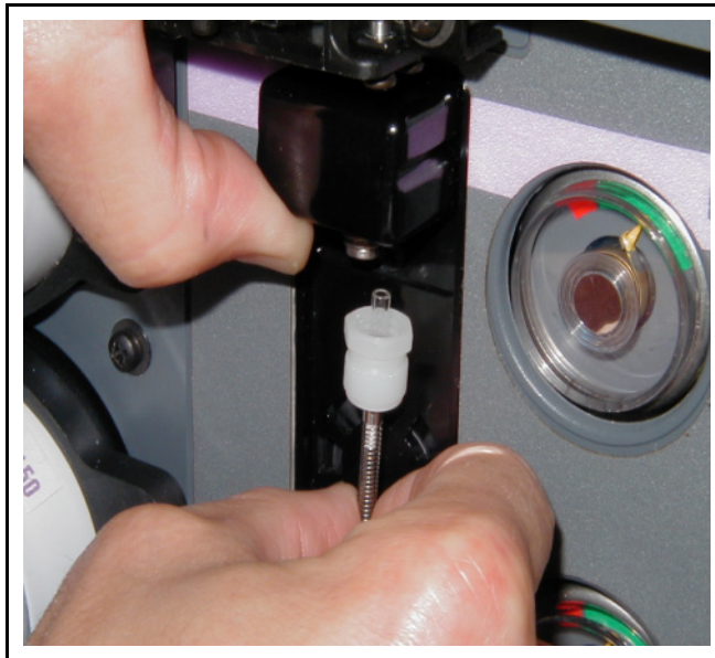
Figure 2-45 Inserting the Top of the Concentrator
