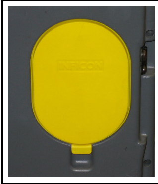
Figure 2-33 Remove the Yellow Plastic Protective Cover on the Bottom of the HAPSITE
