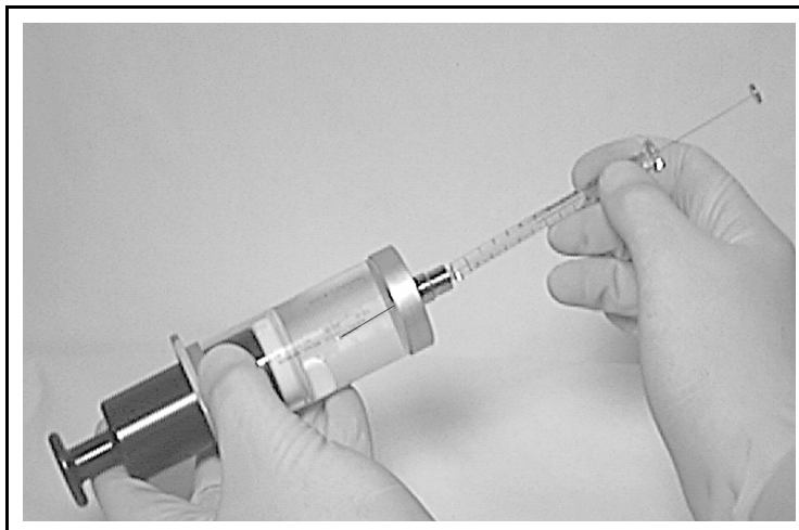
Figure 13-6 Injecting the Mix into the Sample Syringe
