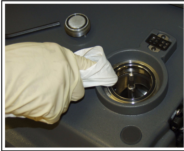
Figure 2-32 Cleaning the Service Module Rubber O-ring using a Lint-free Wipe
