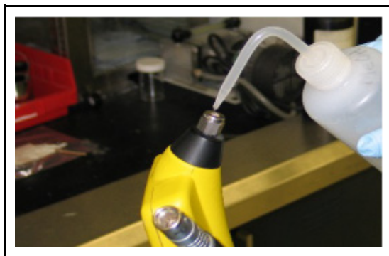
Figure 15-1 Pouring Methanol into Probe and Probe Line
