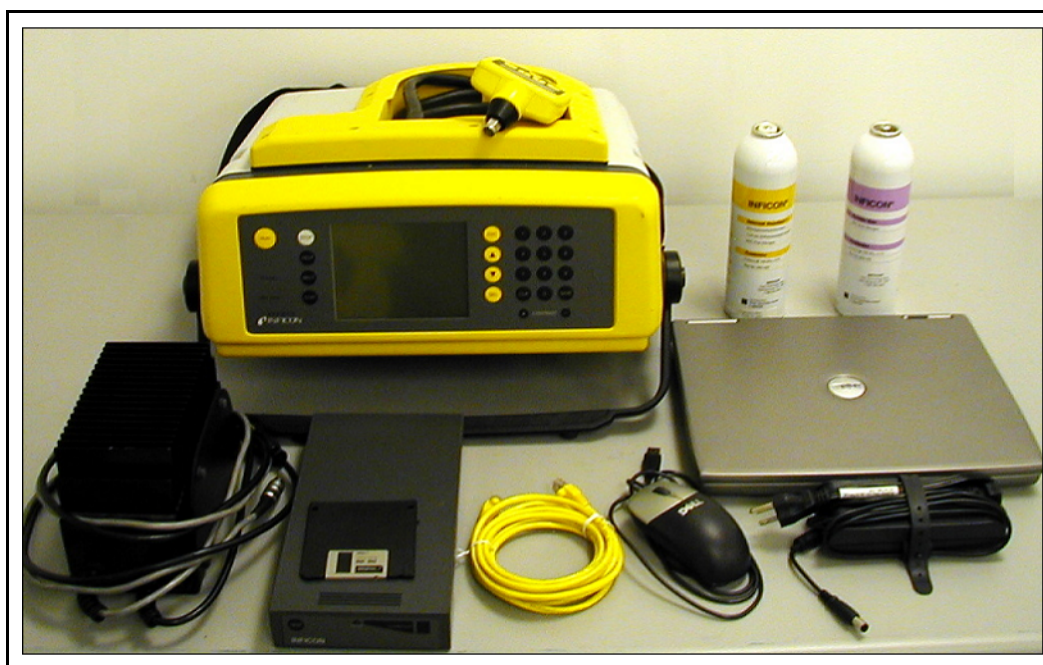
Figure 2-6 HAPSITE Parts for Basic Assembly
