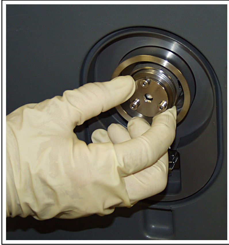
Figure 15-20 Replacing the VI Valve
