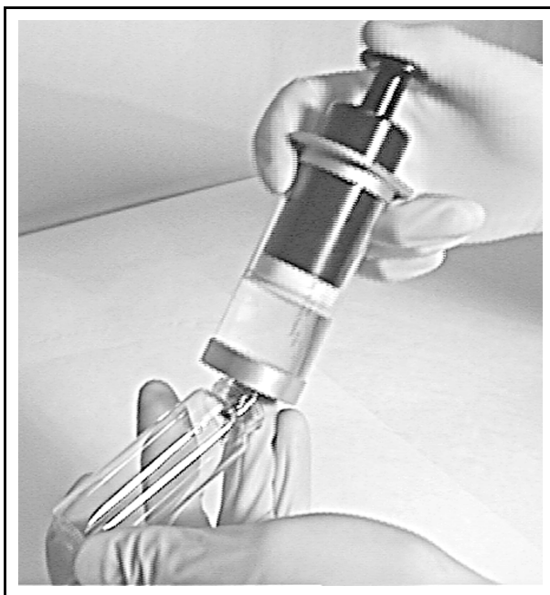
Figure 13-7 Transferring the Sample to a 40 mL Vial
