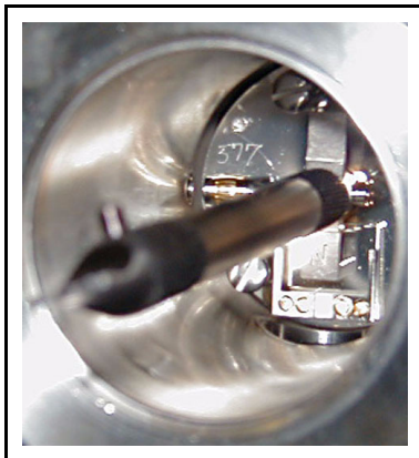
Figure 15-49 Ionizer Removal Tool
