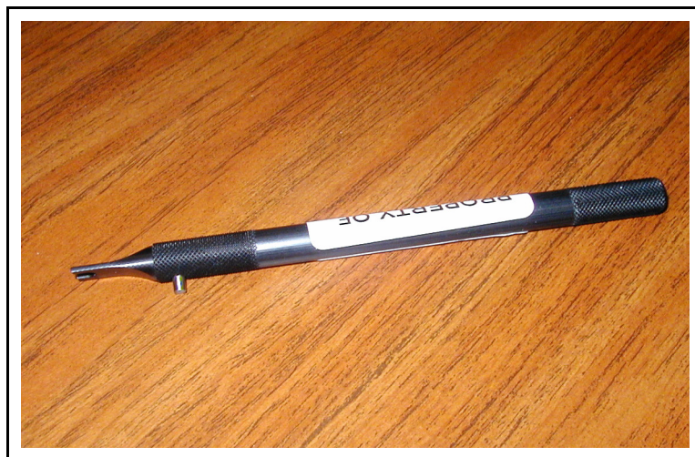
Figure 15-47 Ion Source Removal Tool
