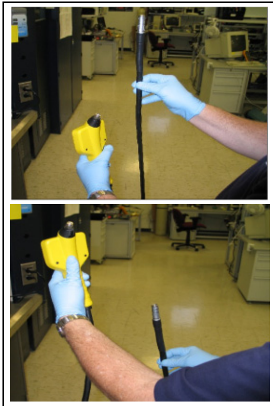
Figure 15-2 Moving Methanol Around in Probe and Probe Line
