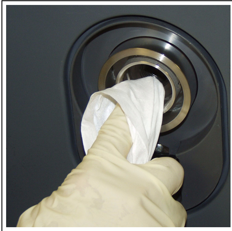
Figure 15-19 Cleaning Bottom of Manifold
