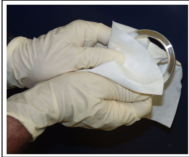
Figure 15-24 Cleaning Aluminum Gasket
