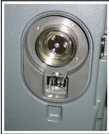
Figure 2-34 Yellow Plastic Protective Cover Removed from the Bottom of the HAPSITE
