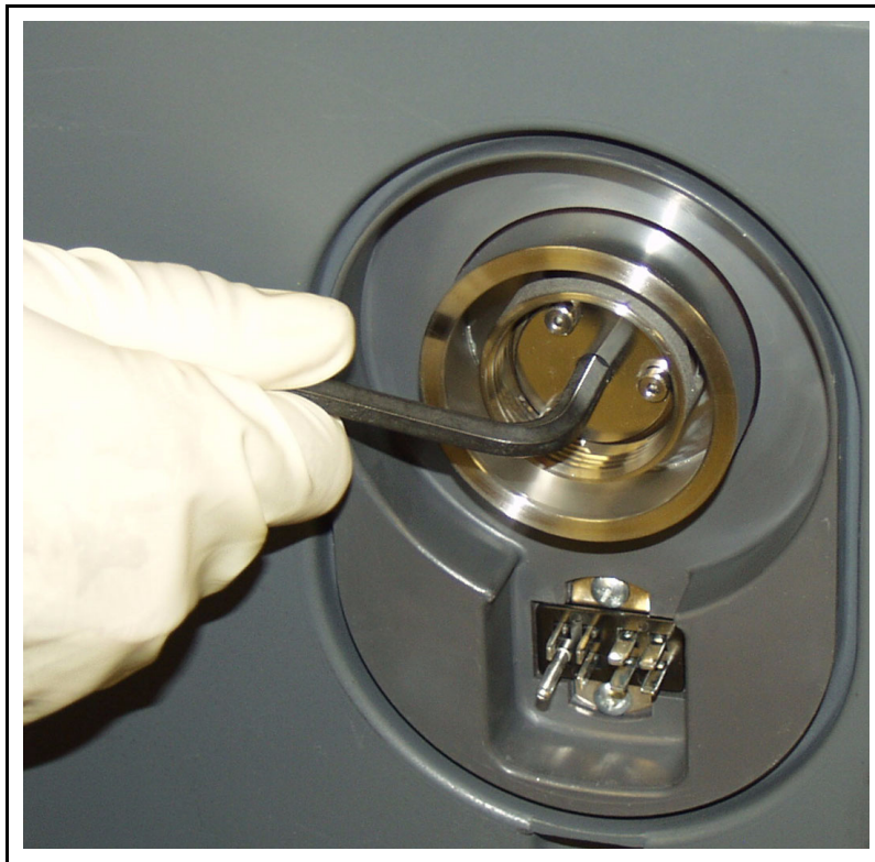
Figure 15-17 Removing the VI Valve
