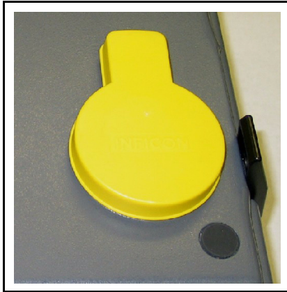
Figure 2-25 Yellow Plastic Protective Cover on Service Module
