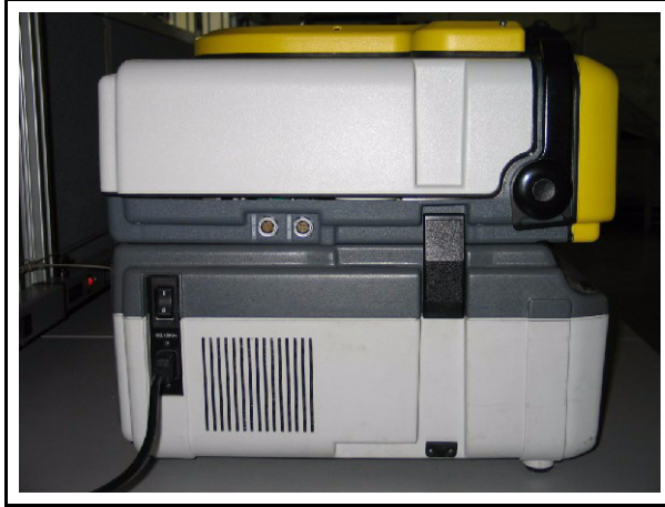
Figure 2-36 HAPSITE Attached to Service Module using Service Module Latches - Left Side View
