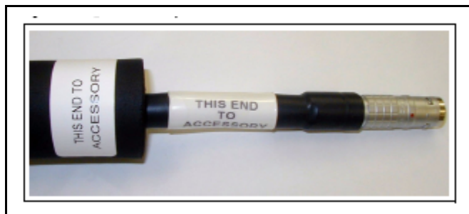
Figure 2-20 Accessory End of the Transfer Line
