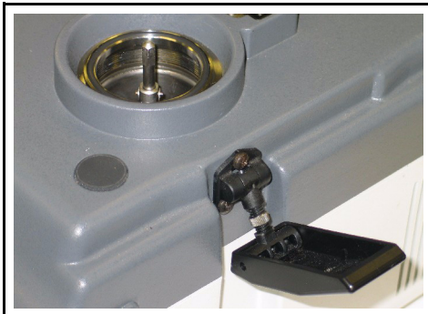
Figure 2-35 Service Module - Showing Latch on Right Side
