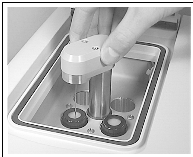
Figure 13-8 Inserting the Needle into a Vial
