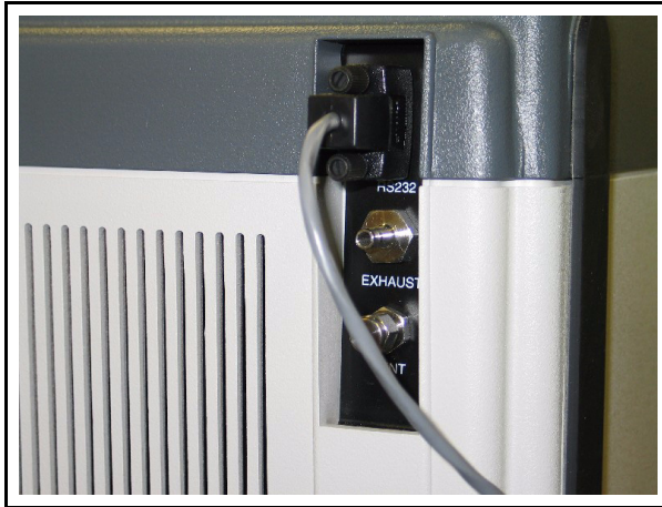
Figure 2-28 RS232 Communication Cable Attached to Back Right Side of Service Module
