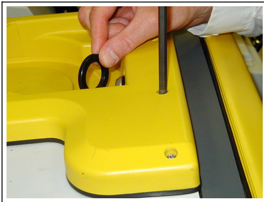
Figure 15-50 Removing Yellow Cover
