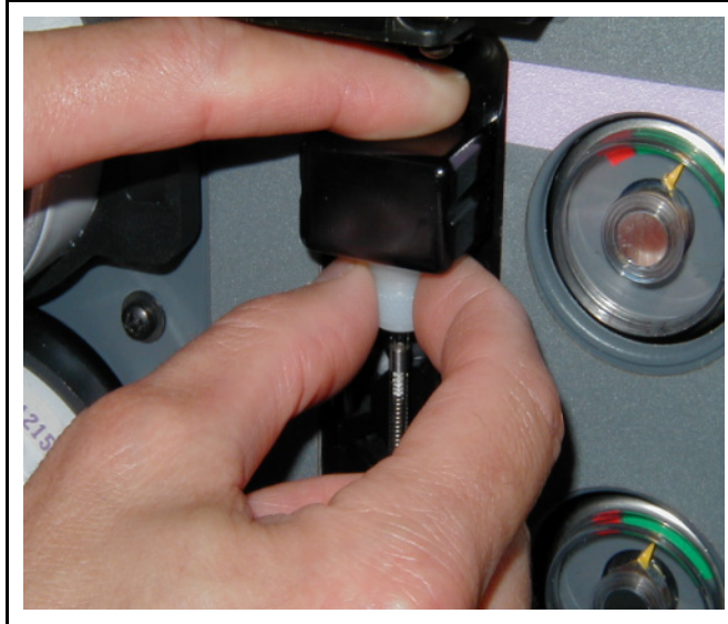
Figure 2-48 Tightening the Top and Bottom Nut
