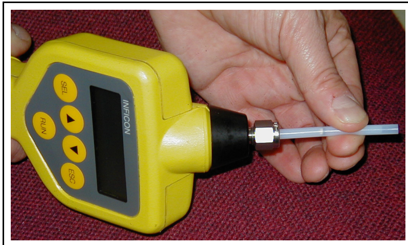
Figure 2-54 Inserting the Swagelok Tube
