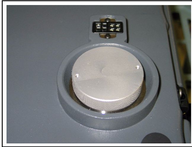
Figure 14-36 Service Module Aluminum Storage Plug in Place on Service Module
