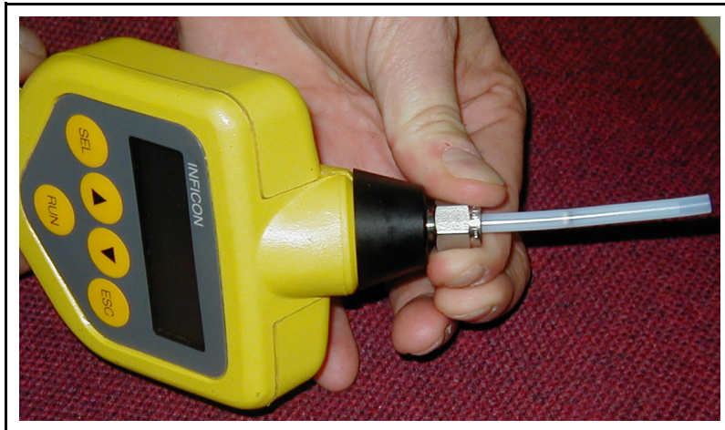
Figure 2-55 Tightening the Swagelok Nut
