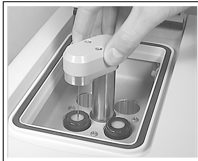
Figure 5-58 Loading the Wells
