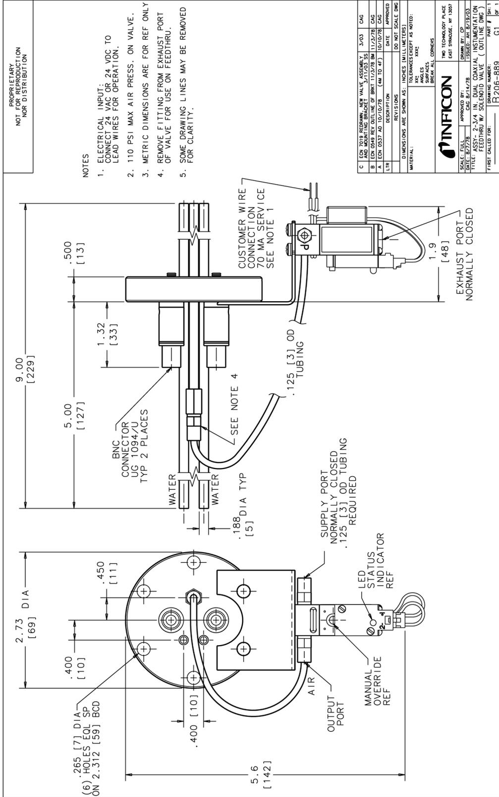
Figure 3-6 CF40 (2-3/4 in. ConFlat) dual coaxial feedthrough and solenoid valve outline
