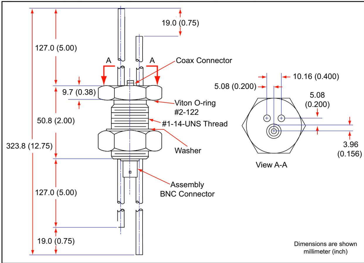
Figure 1-8 2.54 cm (1 in.) bolt feedthrough with three tubes, one coax (PN 750-030-G1)
