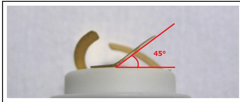
To adjust the prongs on the leaf spring positioned on the ceramic retainer, touch the end of the prong with a gloved finger, or grip the prong with Teflon tweezers, and gently lift it upward. Be careful not to kink the prongs. An ideal bend has a smooth, sweeping shape as shown by [Figure 4-4](#).
