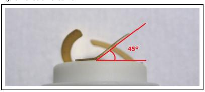
To adjust the prongs on the leaf spring positioned on the ceramic retainer, touch the end of the prong with a gloved finger, or grip the prong with Teflon tweezers, and gently lift it upward. Be careful not to kink the prongs. An ideal bend has a smooth, sweeping shape as shown by Figure 4-4.
