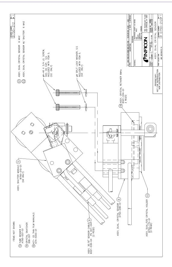
Figure 1-12 PN 750-212-GX dual crystal sensor assembly
