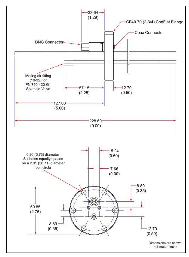
Figure 1-22 CF40 (2-3/4 in. ConFlat) feedthrough with three tubes, two coax (PN 002-080)
