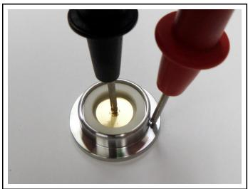
4 Install the crystal holder with ceramic retainer and without the crystal into the sensor. Make sure the crystal holder is held securely in the sensor head cavity. If the crystal holder is loose, refer to section 4.3.4, Replacing the Finger Spring, on page 4-8.
