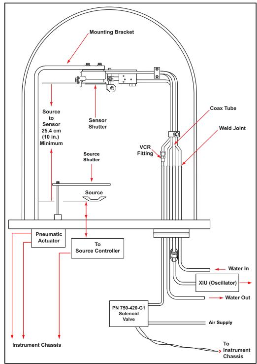
Figure 2-1 Typical UHV Bakeable Sensor installation
