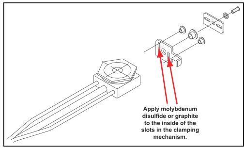
Figure 4-6 Lubricating the clamping mechanism
