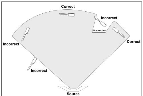
Figure 2-2 Sensor installation guidelines
