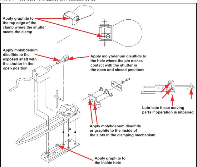
Figure 4-7 Lubrication of shuttered UHV Bakeable Sensor
