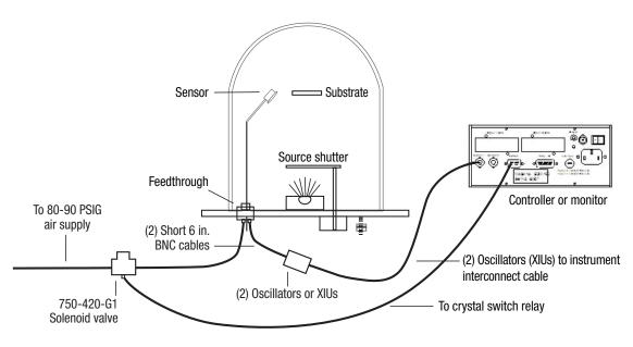
NOTE: (2) indicates that two XIU or oscillator packages are required for a typical dual sensor installation.
