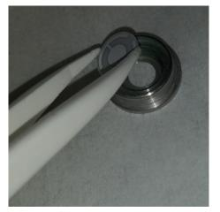
Replace the ceramic retainer. Initially orient the ceramic retainer at an angle to display the spring wire segments in the crystal holder. Avoid using excessive force when handling the ceramic retainer to prevent breakage. Avoid rotating the ceramic retainer after installation, to prevent scratching the crystal electrode.
