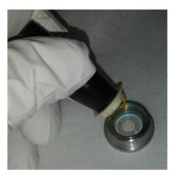
7. Release the crystal snatcher with a slight side-to-side rocking motion. Using the backside of the crystal snatcher, push the ceramic retainer to ensure it is completely seated.
