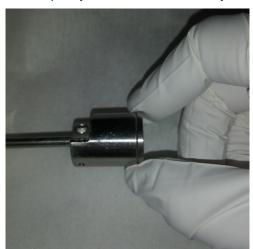
9. Install the QCM sensor back on the foreline with a KF25 clamp and the appropriate centering ring.
