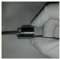
4. Install the QCM sensor back on the foreline with a KF25 clamp and the appropriate centering ring.
