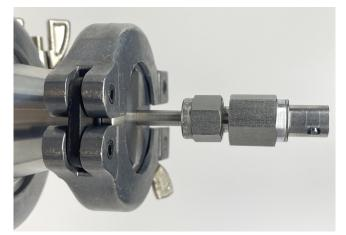
2 Twist the crystal holder counterclockwise to align the locking pin, then pull the crystal holder straight out of the QCM sensor body.
