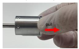
3. Insert the tapered end of a crystal snatcher (PN 008-007) into the ceramic retainer as shown below and apply a small amount of pressure. This locks the ceramic retainer to the snatcher and allows the ceramic retainer to be pulled straight out.
