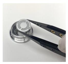
6. Replace the ceramic retainer. Initially orient the ceramic retainer at an angle to display the spring wire segments in the crystal holder. Avoid using excessive force when handling the ceramic retainer to prevent breakage. Avoid rotating the ceramic retainer after installation, to prevent scratching the crystal electrode.
