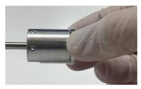
4. Install the QCM sensor back on the foreline with a KF40 clamp and the appropriate centering ring.
