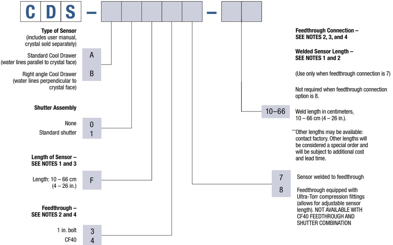
The following combinations are not available: CDS-A1F48, CDS-B1F48. Examples of non-valid part numbers include all options with compression fittings and a welded sensor length; for example, CDS-A0F48-20, etc.
