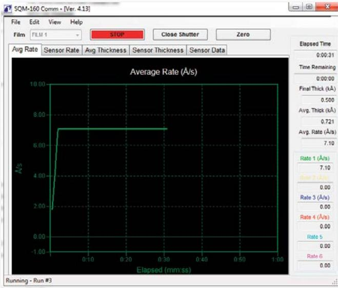
Enhanced software provides a visual display of process data for easy process analysis and documentation. Backup of the SQM-160 setup data allows for process consistency.
