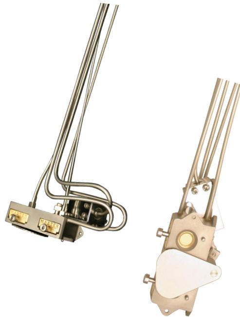
The Cool Drawer Dual Sensor with the CF40 flange is pre-installed in a special two piece 7 cm (2¾ in.) ConFlat® feedthrough. This allows the sensor head to be rotated independently of the flange and circumvents the dimensional limitations of the CF40 flange. Sensor / feedthrough length can be specified between 10 – 66 cm (4 – 26 in.).
