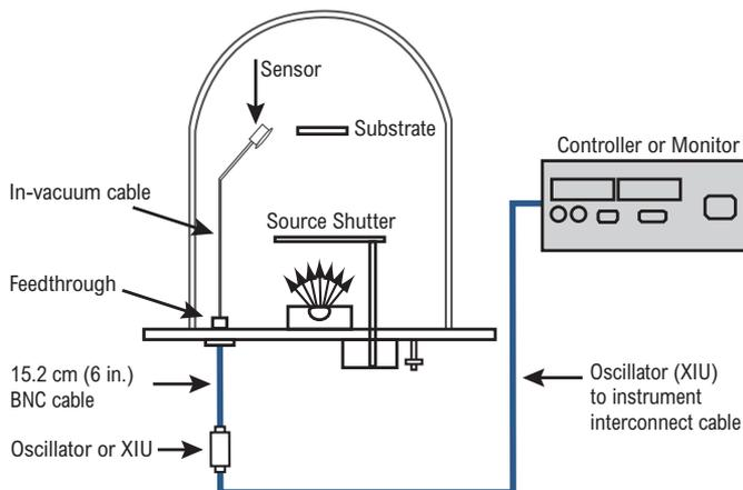
**NOTE 1:** Feedthrough configuration varies depending on options selected (Front Load or Cool Drawer, with or without shutter, type of feedthrough, etc.). Example: SL-A0E37 uses feedthrough PN 002-042 while SL-A1E37 uses feedthrough PN 750-030-G1.
