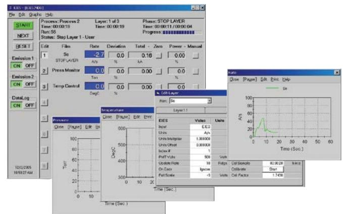
Guardian software provides all of the functions required for a six optical detector, eight output, multi-layer codeposition controller. Process settings, numeric data, and graphs can be displayed during all phases of deposition.
