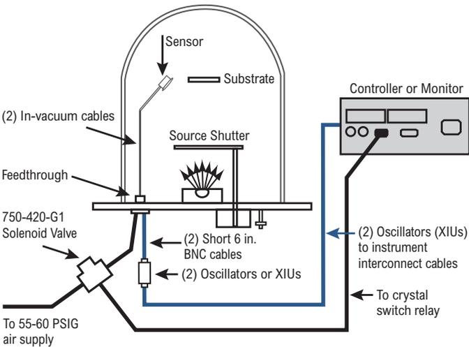
**NOTE:** (2) indicates that two XIU or oscillator packages are required for a typical dual sensor installation. 779-220-G1, crystal two switch option allows operation with only one oscillator (XIU).
