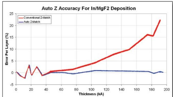
Auto-Z dramatically improves the accuracy of measured thickness for multiple materials and layers.
