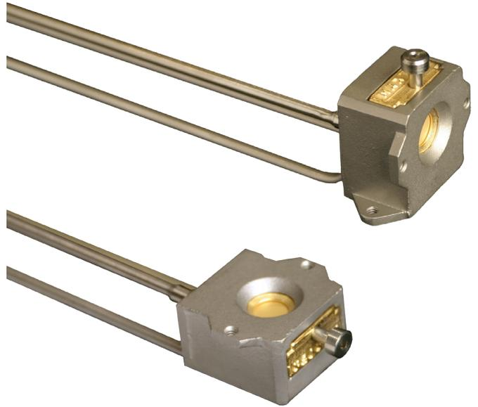
When selected with the welded CF40, the sensor is designed for high temperature processes where reliability is critical. Constructed of stainless steel and ceramic materials it is suitable for applications requiring high temperature bakeout (see specifications).
