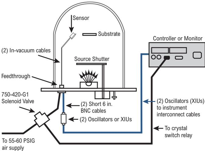
**NOTE:** (2) indicates that two XIU or oscillator packages are required for a typical dual sensor installation.
