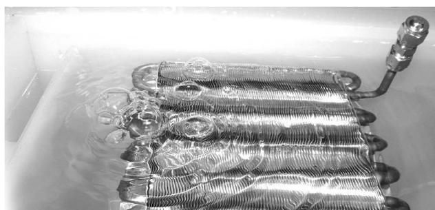
At a leak rate of 0.06 sccm, one bubble per second forms under ideal conditions, but at a leak rate of 0.006 sccm, it takes 30 seconds until a single, small bubble forms.
