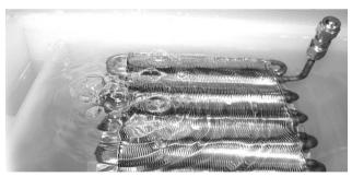
At a leak rate of 0.06 sccm, one bubble per second forms under ideal conditions, but at a leak rate of 0.006 sccm, it takes 30 seconds until a single, small bubble forms.
