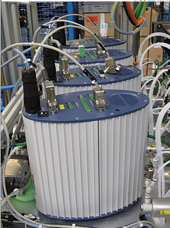
**Robert Bosch's leak-detection test system for bifuel valves has four parallel stations, each of which features a T-Guard detector and a vacuum chamber. Photo courtesy Inficon**
