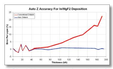
Auto-Z dramatically improves the accuracy of measured thickness for multiple materials and layers.
