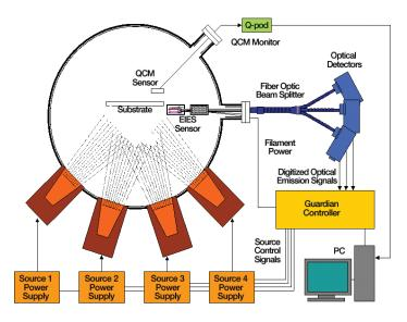
Figure 1: Conceptual system configuration. (See manual for source to sensor alignment requirements.)
