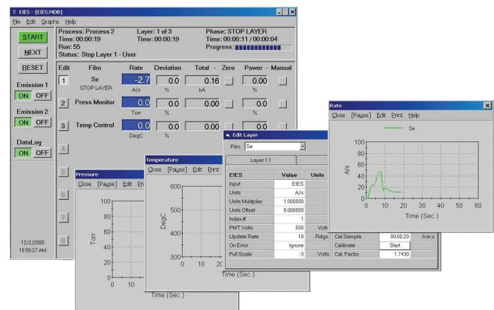
Figure 2: Guardian software provides all of the functions required for a six optical detector, eight output, multi-layer codeposition controller. Process settings, numeric data, and graphs can be displayed during all phases of deposition.
