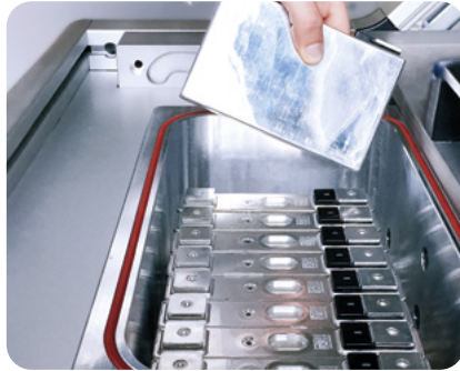
Testing hard case battery cells in a vacuum chamber.
