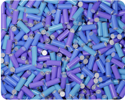
Scrapped round cells from an assembly line for lithium ion batteries.
