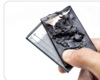
Fire damage to a lithium-ion battery.
