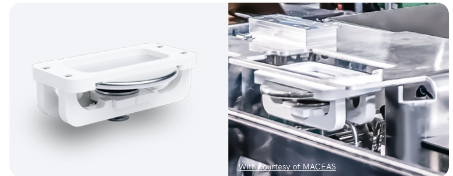
Calibration of the ELT battery leak detector family with a certified E-check calibration leak.
