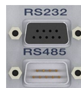
DE-9 Connectors for connections to user supplied cables for serial communication port – DE9P (RS485), DE9S (RS232)
