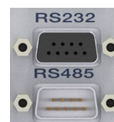
DE-9 Connectors for connections to user supplied cables for serial communication port – DE9P (RS485), DE9S (RS232)
