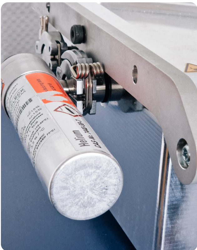
连接至泄漏检测腔室的校准漏孔
