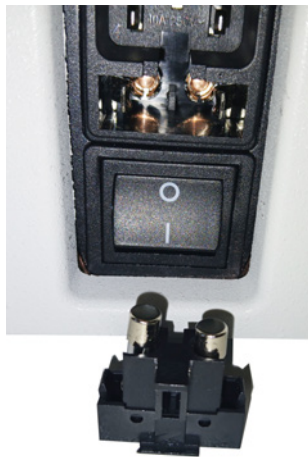
Fig. 12: Cover with fuses
