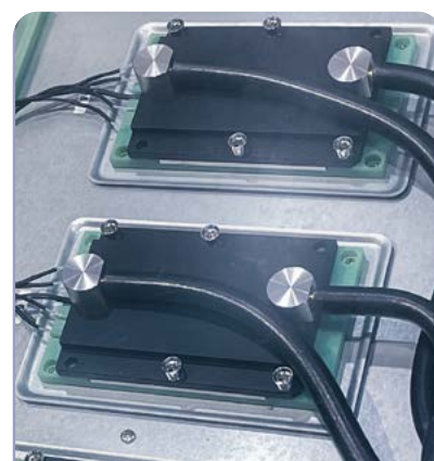
Prototype of a direct-to-chip cooling design. Components to be tested for leaks include, among others, cold plates, pipes, and quick connectors.
