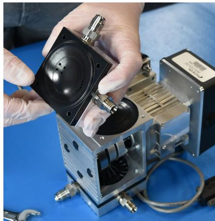
**6** Separate the diaphragm plate from the head cover.
