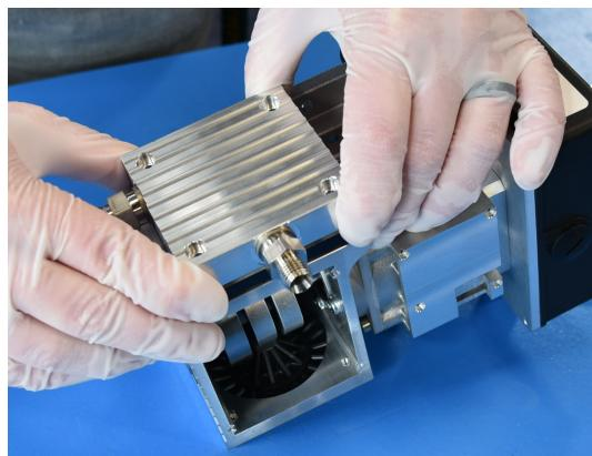
**16** Replace the four hex screws to secure the head cover. Perform the steps again for the second pump head. Replace the cam cover and interstage tubing.
