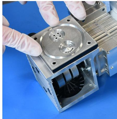
**14** Install the new valve disks, valve seals, and the O-ring into the diaphragm plate.
