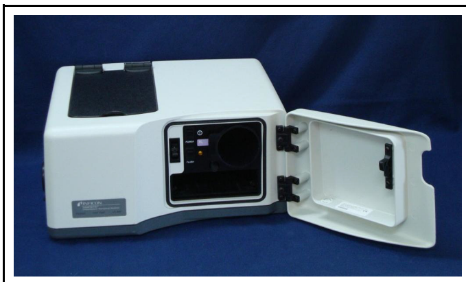
Figure 3-10 HSS Front Door
