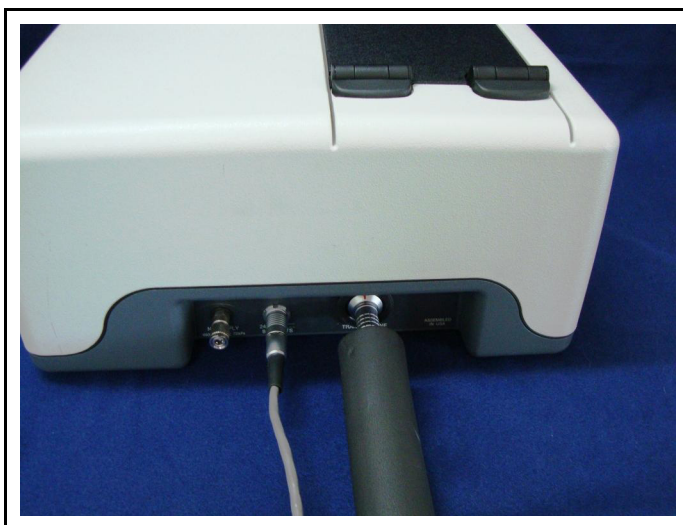
Figure 3-9 Inserting Transfer Line
