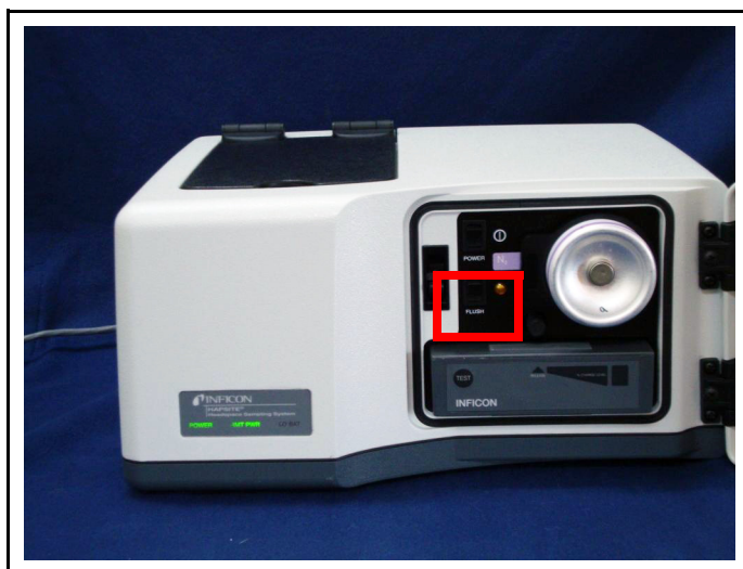
Figure 5-1 Flush Switch Inside The HSS
