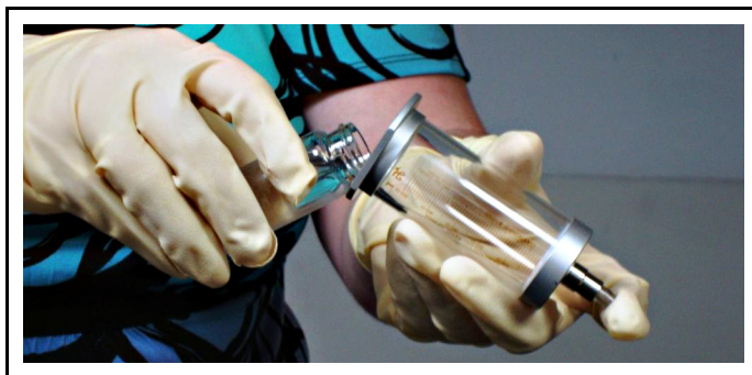
Figure 3-15 Transferring the Sample into a Sample Syringe
