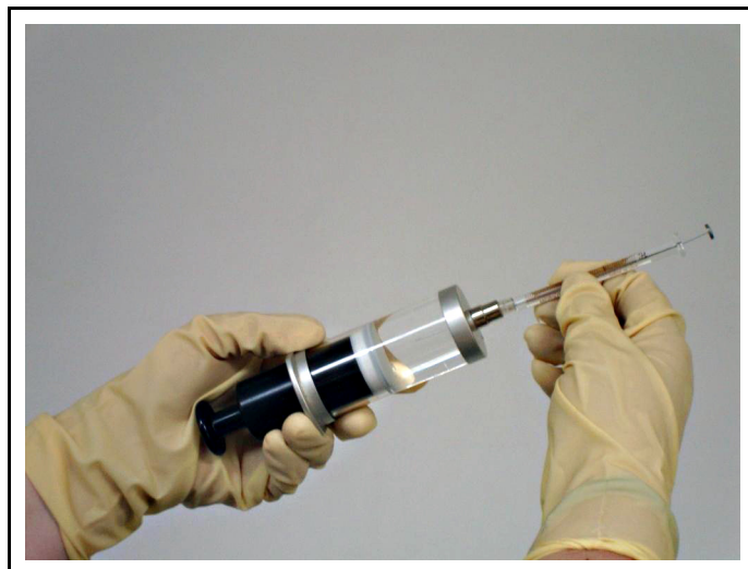
Figure 3-17 Injecting the Mix into the Sample Syringe
