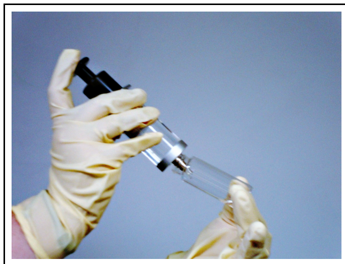
Figure 3-18 Transferring the Sample to a 40 mL Vial
