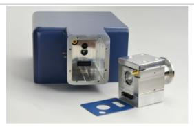
6 Install the new inner gasket from replacement MSC kit. If a new inner gasket is not available, reuse the original inner gasket. To install the inner gasket, place Quantus LP100+ upright on the work surface so that the gasket can rest at the bottom of the cavity. Leave Quantus LP100+ in this upright position for the next step, installing the new MSC.
