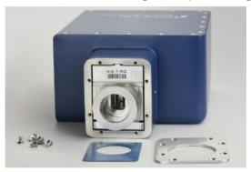
**4** Using a 2 mm hex driver, remove the four (4) set screws (two on each side) holding the MSC in place.
