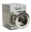
Quantus LP100+ creates a plasma by coupling energy into the gas utilizing a patented planar antenna in the MSC. The antenna is protected by a sapphire window so it is not exposed to the process chamber or gas sample. This provides the LP100+ its unique operating capabilities that allow the sensor to operate in corrosive and aggressive environments. The planar antenna is built using PCB techniques that provide tight tolerances and high performance. The MSC can be replaced in the field.
